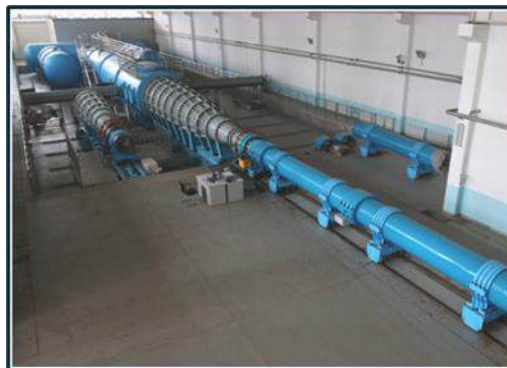
Figure 10 – CAS IOM JF-12 Shock Tunnel, Duplicating Hypersonic Flight Conditions at Mach 5 – Mach 9
